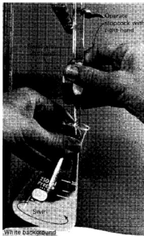
Figure T.16i Titration technique for left-handers.
