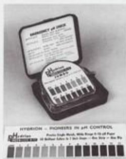
Figure T.17c Test papers impregnated with a mixture of acid-base indicators can be used to measure the approximate pH of a solution.
