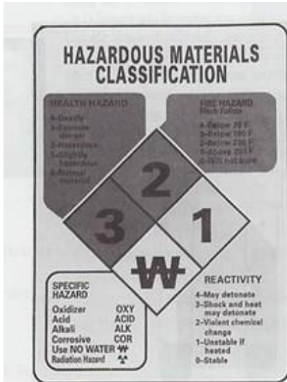
Figure T.3b Hazardous materials classification system.
